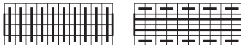
Fig. 2. Wires transporting the false (the left one) and the true signal (the right one).
